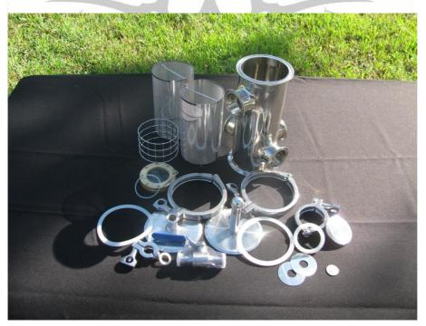
**Figure 1: SD Gin Head Supplied Components**
