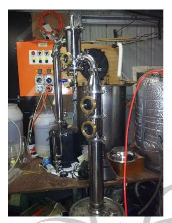
Figure 10: The Authors SD Gin Head adjusted to height using a 510mm section and 2 empty bubble Tees
