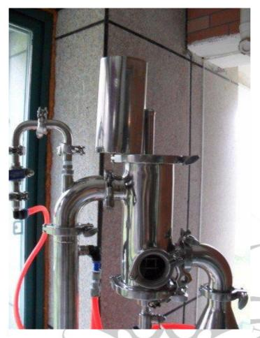
Figure 12: Standard Configuration with optional threaded 90° for clean in place
