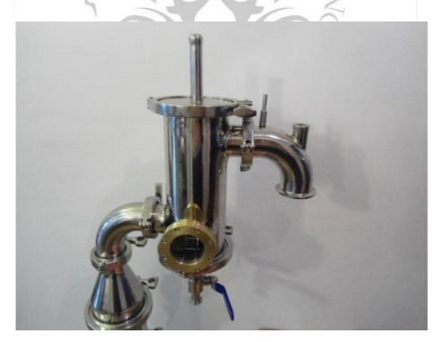
Figure 11: Assembled SD Gin Head with optional cleaning port on  $90^{\circ}$  elbow
