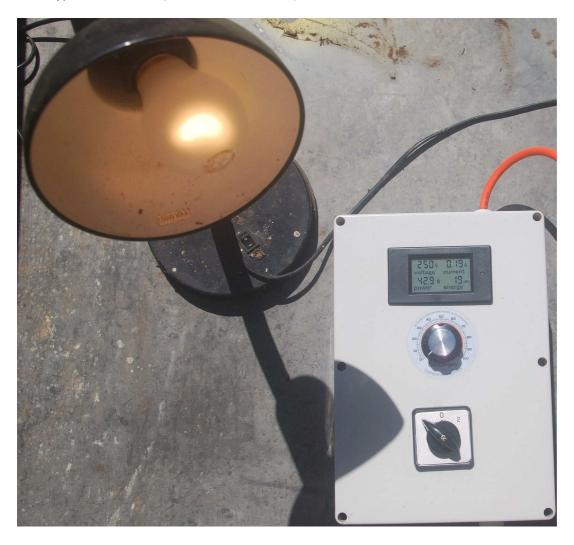
With current going through the SSR [via switch position '2'], and the StillDragon potentiometer set at 0%...well we get 1.8W – all being consumed by the SSR.
