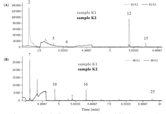
Figure 3. Chromatograms of Czech vodka samples K1 and K2: (**A**) a record of the characteristic ion (m/z 88) of ethyl esters of carboxylic acids, (**B**) a record of the ion (m/z 81) of substituted furans; the peak numbers in the chromatograms correspond to the compounds listed in Table 4
