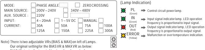
BIAS (Output adjustment of basic voltage) ..... 6mA MAX (Max. Output adjustment) ..... 0~100%
