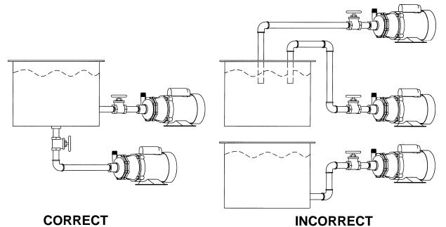
12. Suction Pressure: Systems utilizing high suction pressure where a pump is used to boost system pressure is of concern. Be sure that the pressures do not exceed that of pump design, otherwise severe damage and possible operator injury could result.
